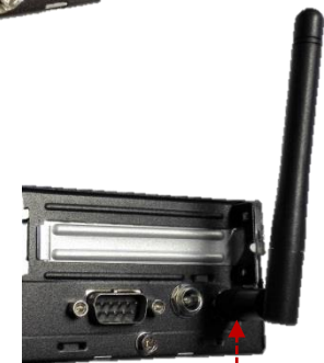
WLAN antenna installed (consumer option)
