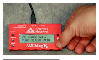
Newer systems feature support for AMI Debug Rx, a USB connected alternative to the PCI POST Card. AMI Debug Rx is a low-cost debug tool built around the debug port feature common to today's USB 2.0 EHCI controllers.
