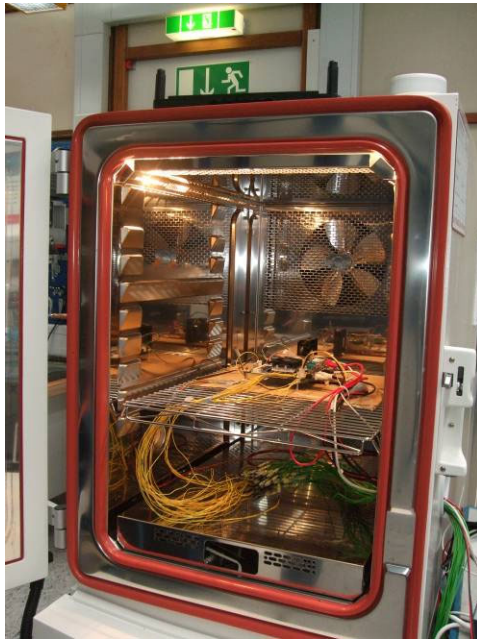
Picture no. 5: EUT in climatic cabinet
