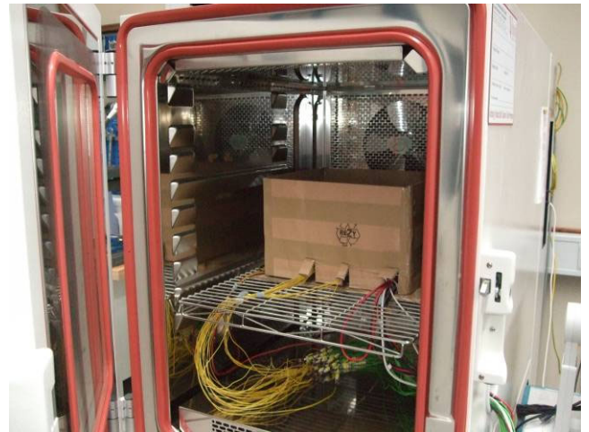
Picture no. 6: EUT in climatic cabinet prepared for measuring
