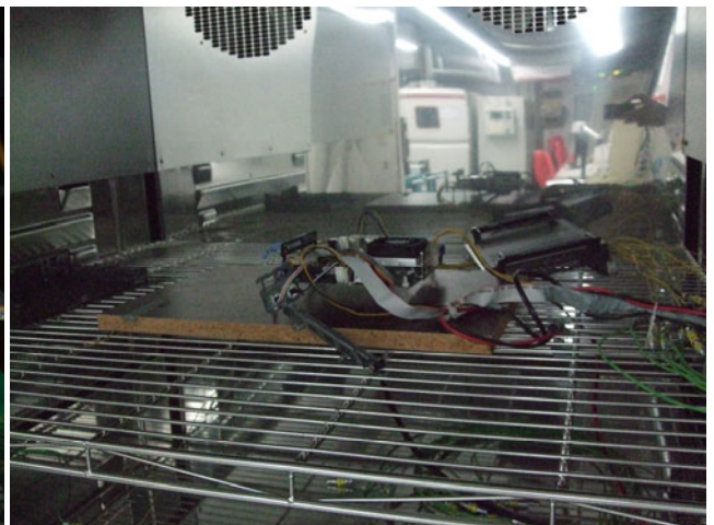
Picture no. 12: EUT without chassis in climatic cabinet
