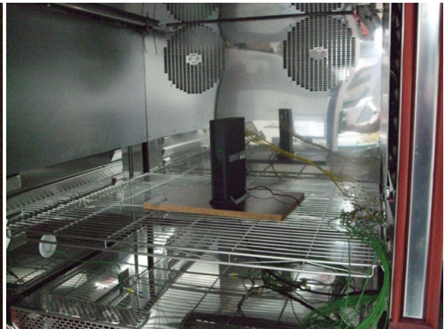
Picture no. 10: EUT in chassis in climatic cabinet
