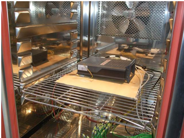
Picture no. 11: EUT in climatic cabinet
