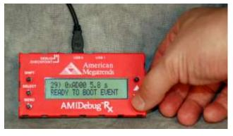
Newer systems feature support for AMI Debug Rx, a USB connected alternative to the PCI POST Card. AMI Debug Rx is a low-cost debug tool built around the debug port feature common to today's USB 2.0 EHCI controllers.
