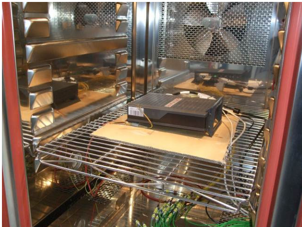
Picture no. 11: EUT in climatic cabinet
