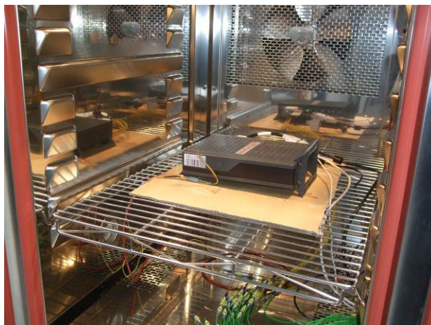
Picture no. 11: EUT in climatic cabinet
